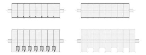
Figure 1 Technical drawing of dowel laminated timber
