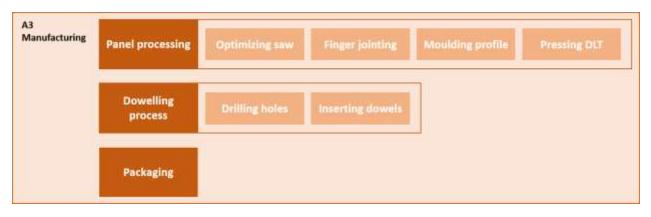
Figure 4 Manufacturing process
