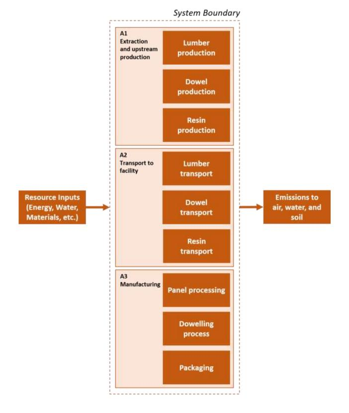
Figure 2 Cradle-to-Gate DLT production flow diagram
